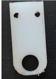
4 movable bearings in Rilsan
