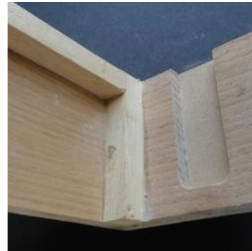
2 guides for movable bearings. Wood has been chosen to be easily glued on the box side also in wood
