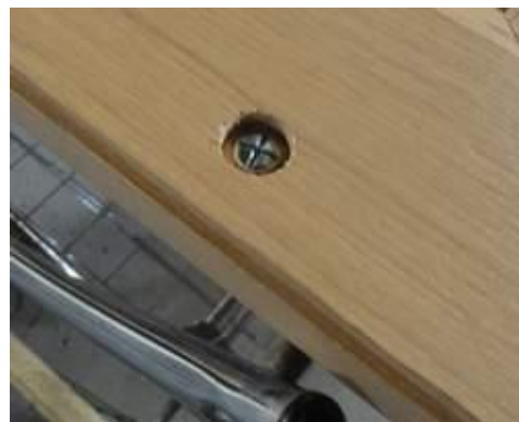
A board is permanently fixed on the tubes - heads must be drowned
