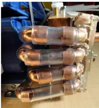
Connecting plastic tubes on each side of the valves unit
