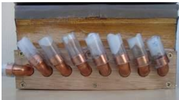
Air outlet at the rear of the blower (on the lower throat).
