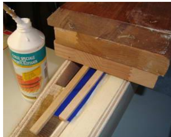
Apply a weight on the skin during drying
