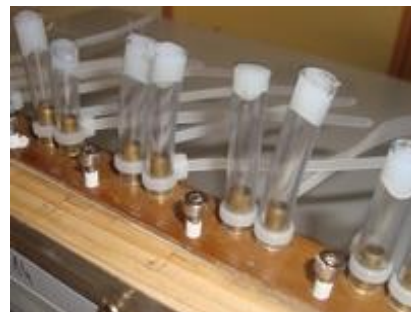
Occultation tubes with caps (plastic pipe + glue gun)
