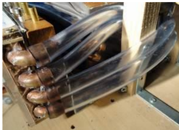
Connecting plastic tubes on each side of the valves unit
