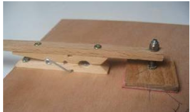
Sketch and photo of the pressure relief valve
