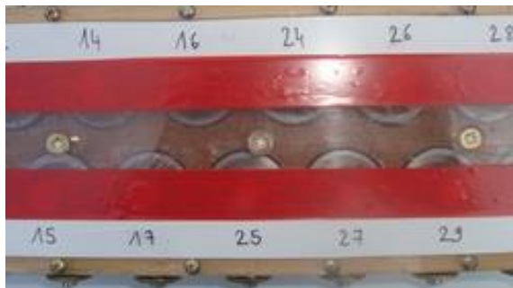
Occultation of holes on the lid by scotch tape.
