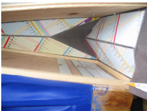
Two stiffeners for front side reservoir
