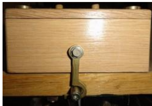
A latch is set on the front panel to ensure a good pressure.
