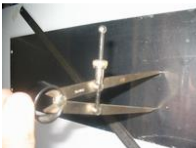
Tracing the form on the aluminum plate
