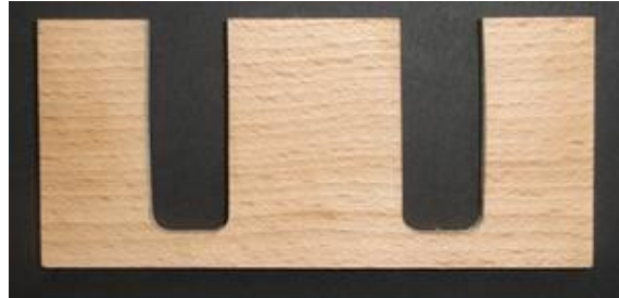
2 guides for movable bearings. Wood has been chosen to be easily glued on the box side also in wood
