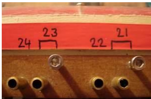
Marking the arrival of the tracker bar and adjusting screws (repetition speed)
