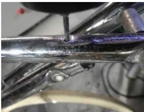
The horizontal tubes are drilled for receiving screws.
